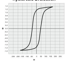
EP-400 is designed to measure AC magnetic properties of flat rolled magnetic materials at high frequency by using Watt-meter, Ammeter, Voltmeter and Source. Epstein bridge test method is a fundamental method for evaluating the magnetic performance of flat-rolled magnetic materials in either sheared or stress relief annealed condition. This test method is suitable for design, specification acceptance, service evaluation, and research and development.
