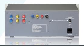
LCD780 is multi-range power Analyzer with basic 0.07% R+R accuracy. 8 range of voltage, 8 range of current and total 64 range of power and power factor gives more accurate result. The gap less four-quadrant power measurement technique gives better accuracy at distorted waveforms or AC drive (VFD) operated power supply.
