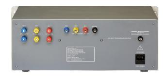
DXL780 is suitable for transformer & motor testing. It has 8 range of voltage & 8 range of current which is Auto or manually selectable. User interface by 22key become more easy and understandable. And the most efficient programming technique used to implement FIR & IIR filter that gives steady result and option of selectable display update rate.
